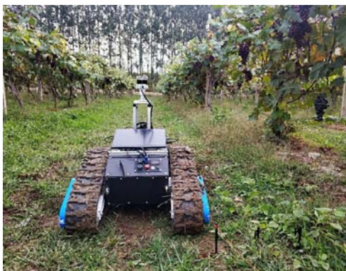
Figure 4 The robot collects three-dimensional point clouds in the vineyard
