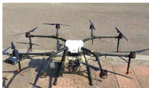
Figure 1 MG-1P four-rotor electric unmanned aerial vehicle (UAV) sprayer
