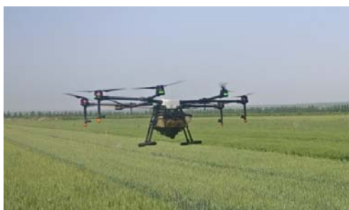
Figure 1 MG-1P four-rotor electric unmanned aerial vehicle (UAV) sprayer
