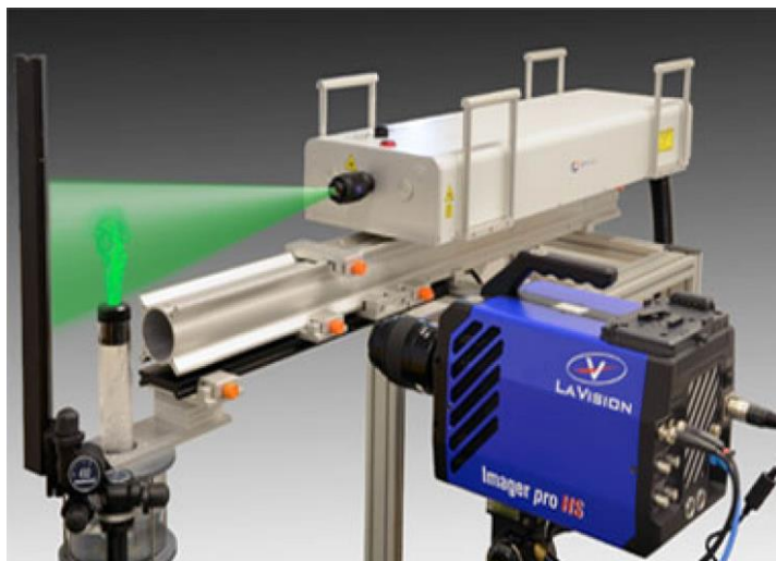
a. Particle image velocimetry
