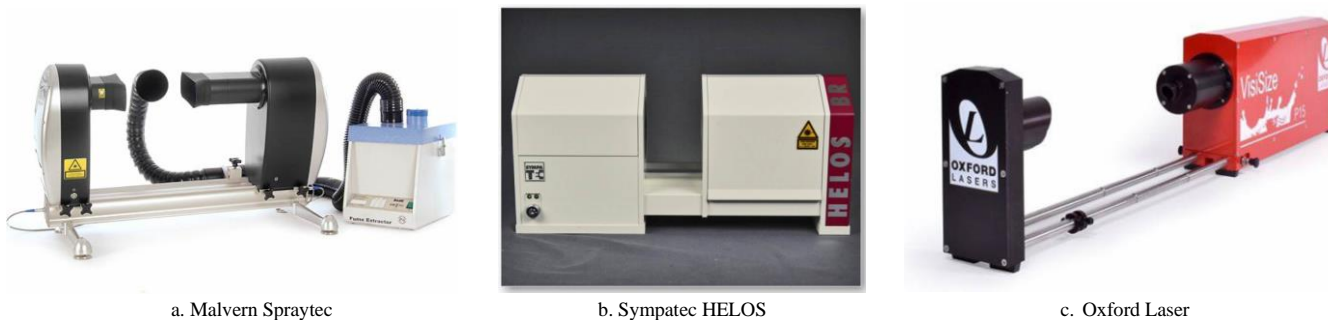
Figure 8 Main brands and models of laser particle size analyzer
