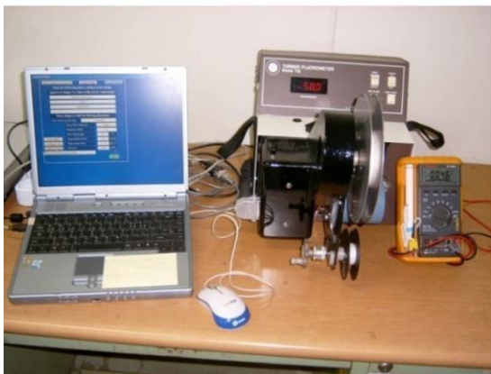
Figure 6 The WRK string analysis system detecting fluorescence level of rhodamine B (WT)
