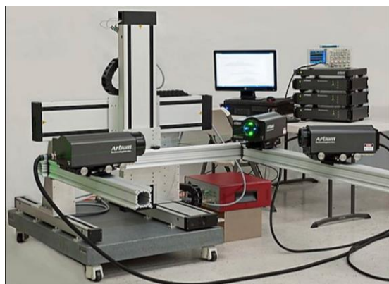
a. Phase Doppler Interferometer
