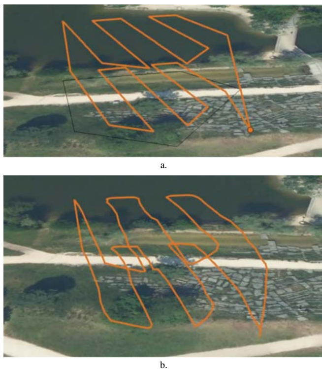
Figure 7 (a) Pre-set planned route and (b) UAV simulation environment flight path
