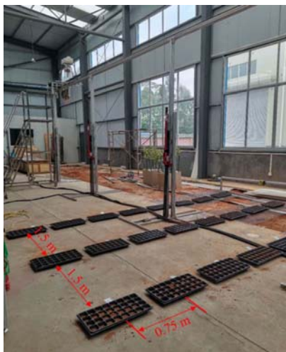
Figure 12 Schematic diagram of the layout of the seedling tray for the sowing test
