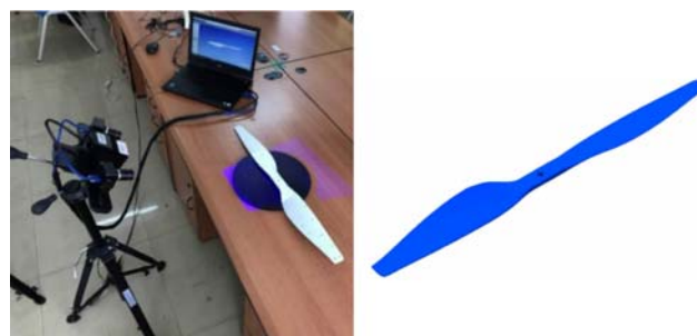
a. 3D scanning b. The 3D model of rotor Figure 1 The 3D scanning process of rotor
