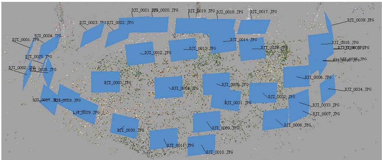
Figure 4 The position of the camera
