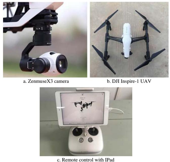
Figure 1 The UAV system
