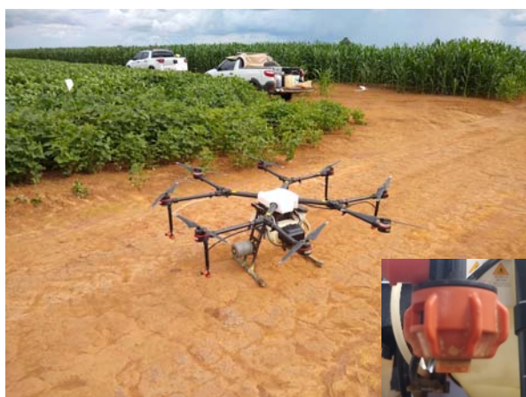
Figure 1 Unmanned aerial vehicle (UAV) used in the experiments; the XR 11001 nozzle in detail (inset).
