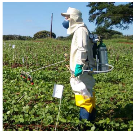
Figure 2 CO 2 -based constant pressure backpack sprayer used in ground application.
