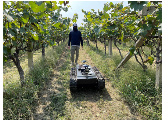
Figure 5 The robot collects three-dimensional point clouds in the vineyard with a running person at the front of the moving robot
