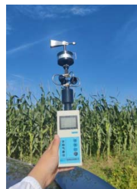
Figure 7 Wind speed and direction meter
