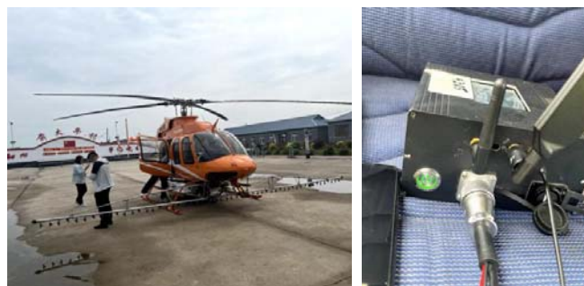
a. Helicopter spray rod b. Monitoring equipment Figure 4 Helicopter spray rod and Monitoring equipment
