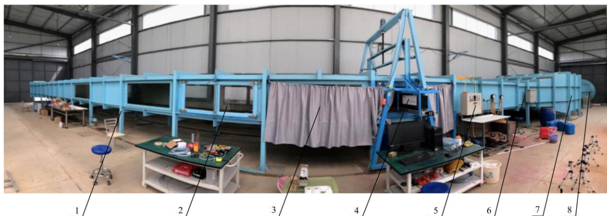
1. Mounting bracket 2. Observation window 3. Test section 4. Droplet size test system 5. Spray system 6. Contractive segment 7. Steady section 8. Drive section
