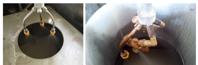
b. Discharge through CCO plates during test
