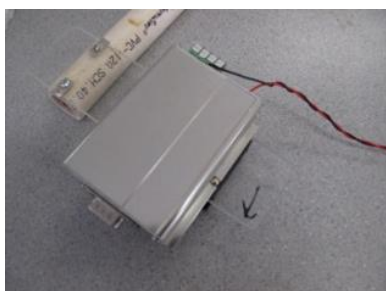
Figure 4 Data acquisition box
