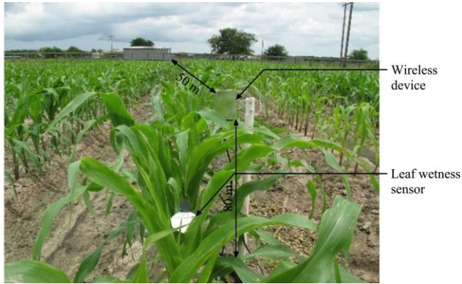
Figure 6 A Smart Sensor node with LWS installed in the USDA College station a few days after planting of corn
