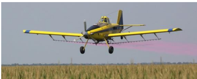
a. Air Tractor AT-502B is powered by a turbine engine and has a 1893-L capacity hopper. Typical application speed is between 58 and 65 m/s
