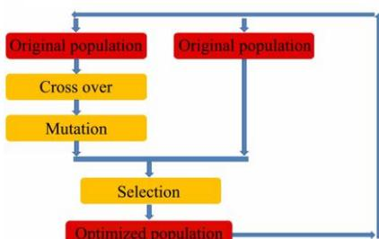
Figure 7 The workflow of genetic algorithm
