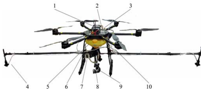
1. Power 2. Wind pressure transducer 3. Microcontroller 4. Sprinkler 5. Pesticide box 6. Solenoids valve 7. Micro diaphragm pump 8. Camera 9. Pan-tilt 10. Flow sensor
