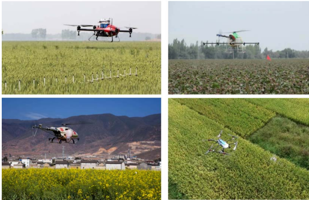
Figure 5 Plant protection UAVs spraying for different crops
